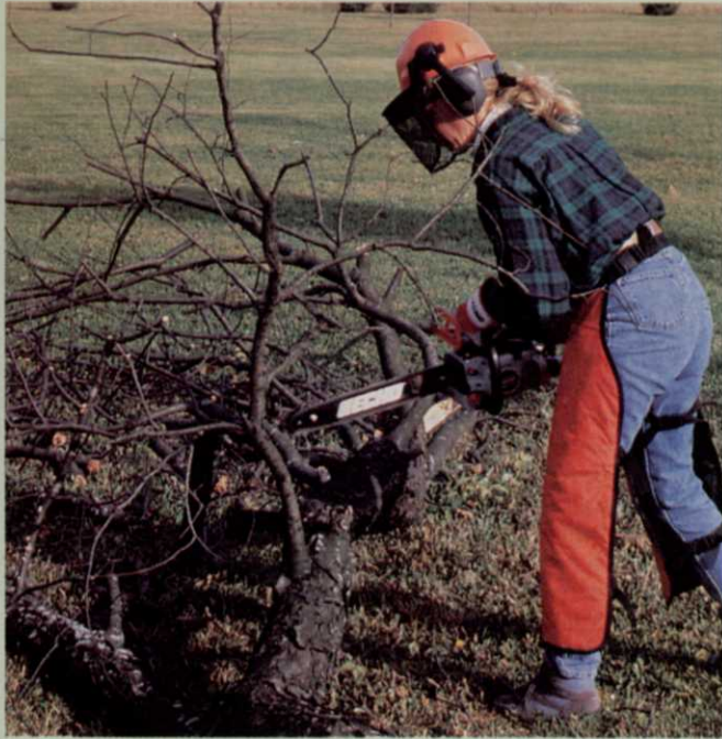
Echo saw is powered by a 33.4 cc, two-stroke engine. Some saws have chain guards. Operator should stand on the side of the trunk opposite the limb being cut.
