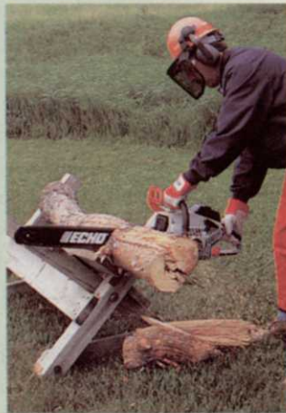
Be aware of the direction the chain will go if it breaks.
