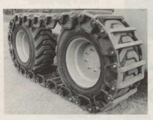
for convenient field replacement; more floatation. These skid steers are easy to install with the new installation tool.
