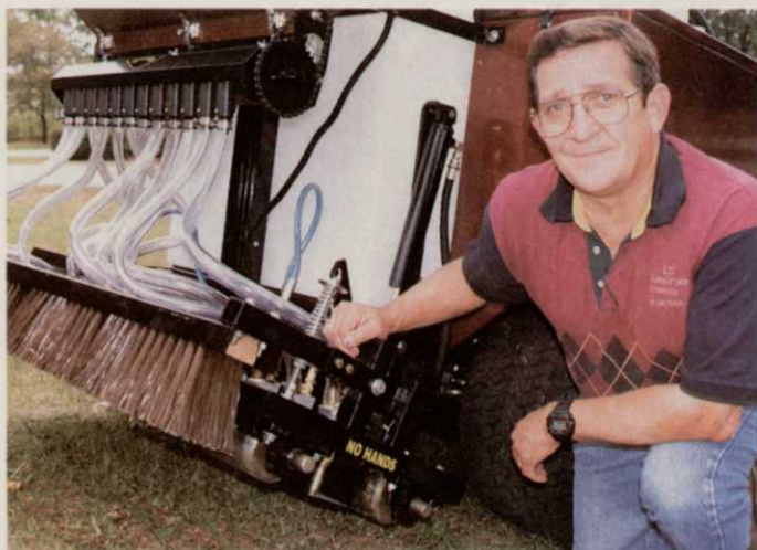
Don Taylor, president of LIS, Inc., Crystal River, FL, developed the SGI after years of working with high-pressure water for industrial uses. He says SGI can be used to apply granular or liquid.
