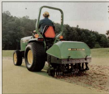
Deep-tine aerification can be incorporated into a core cultivation program for faster results.
