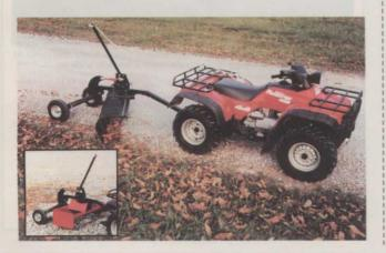
pull lever to raise the unit while turning or dumping and a clevis-type hitch.
