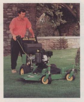
This unit can be equipped with a 48-inch or a 36-inch deck. The 36-inch deck features two-spindle, timed blades for a superior cut, a larger discharge opening and a new discharge chute for better grass clipping distribution, %-inch to 4 ½-inch cutting height range, and a fixed, deep-deck design.
