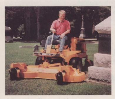
Excel says the 2500 Compact has "the world's fastest edger attachment." The mower turns within its own length on counter-rotating, independent-drive wheels.
