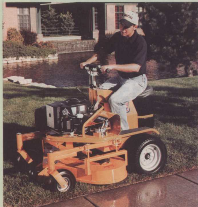
The operator can stand or sit to operate the Hustler ShortCut zero turn rider. Hustler Bar Steering can be mastered in minutes.
