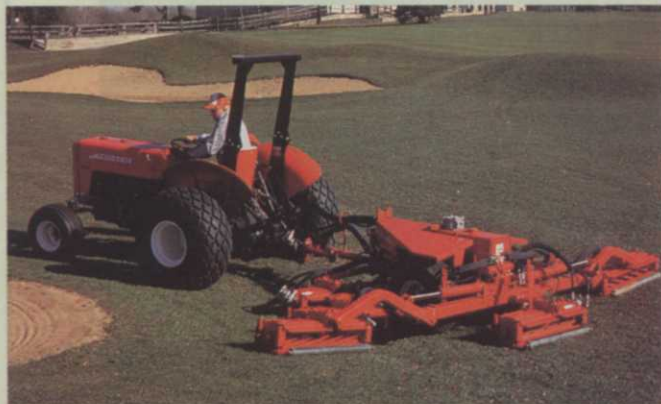
Jacobsen Hydraulic Rangers available in 7-gang or 5-gang versions. The 7-gang model has a 15-foot cutting width.
