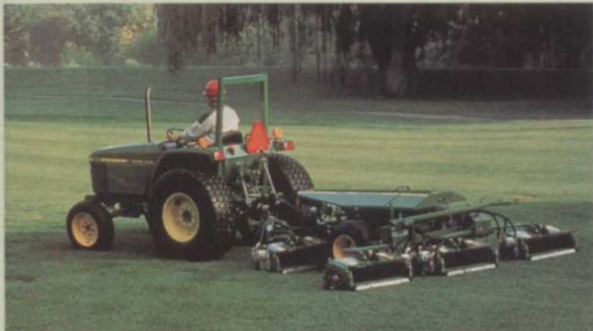
John Deere offers five hydraulically powered 30-inch ESP reels on the JD 365 hydraulic gang mower. Cutting width, 134 inches.
