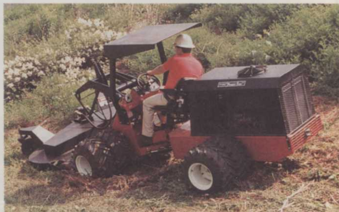
Power Trac 45-degree slope mower has a low center of gravity and wide wheel base, keeping it grounded on steep terrain.
