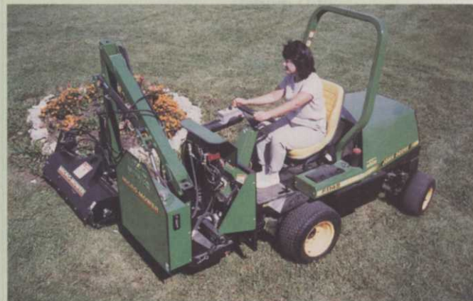
The MicroMower line from R.L. Parsons & Sons consists of four models designed for tractors in the 15 hp to 35 hp range.
