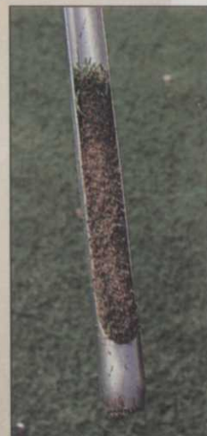
The soil sample reveals soil layering characteristics, possible compaction, and soil nutritional needs.
