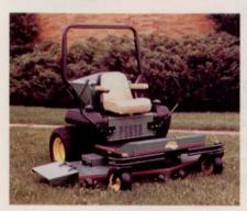
It features a 72-inch cutting width with forward travel speeds up to 9.5 mph. Other features include: electronic deck lift and height adjustment system, large tires and wider wheelbase, easy service access, and optional ROPS.
