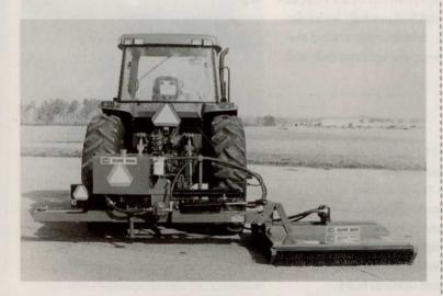
ciently," said Robert O. Moore of Bush Hog. The SM-60 delivers a 5-footwide cut with a maximum reach of the cutter head of 12 feet from the tractor center line. Operation is all hydraulic.
