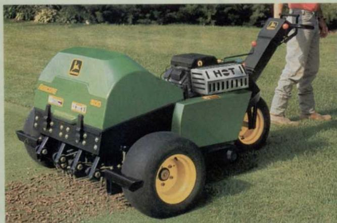
John Deere's 800 walk-behind Aercore features a heavy-duty frame, tine rams, and adjustable operating speeds.
