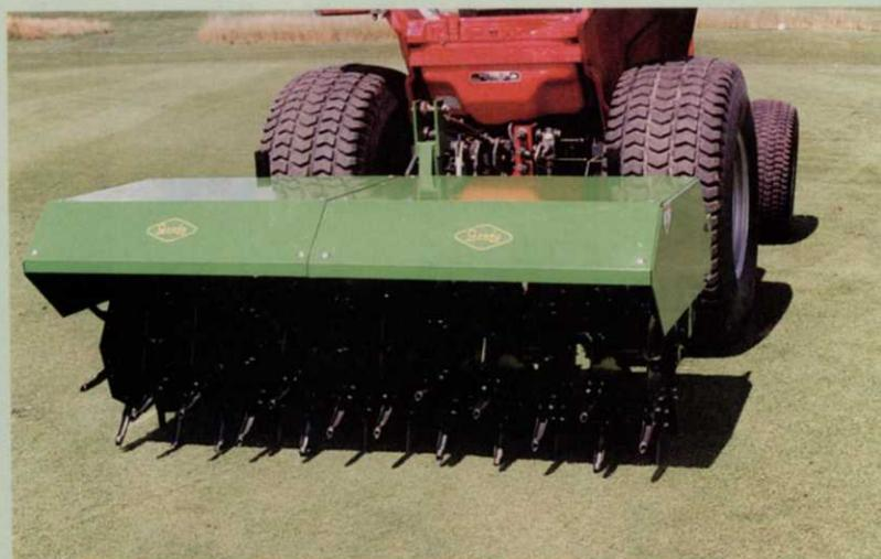
Gandy Models 4972 and 4996 feature dual-wheel aerating heads which independently follow ground contour. Both mount on Category One 3-point hitch.
