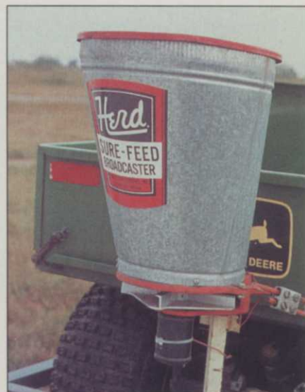
Mounted broadcast spreaders cut worker exposure to pest, cover ground faster.
