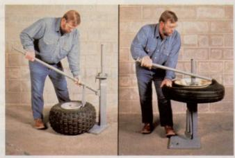
breaker, mount/dismount bar and a tire repair wall chart. Additional accessories available include; a small tire tool for smaller turf-type tires, an ATV bead breaker and a tire spreader to inspect and repair tire damage.
