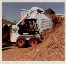
gate. The 751 also has a bigger starter and battery and a slower engine RPM. The 753 has a larger tilt cylinder and more rollback power, more hydraulic flow and faster travel speed (up 10%
