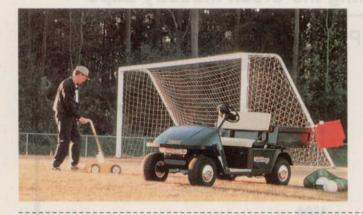
The unit also has rack and pinion steering and a heavy-duty cargo bed-liner. Optional equipment is also available, such as, a cab with doors, flatbed, lights, power dump bed, all-weather enclosure etc. The gasoline powered version has a 9 hp, 295 cc, twin cylinder, overhead cam engine; an automatic, continously variable transmission and a six gallon fuel tank. The electric version has a heavy-duty, 36 volt, high efficiency motor for quiet, powerful operation.
