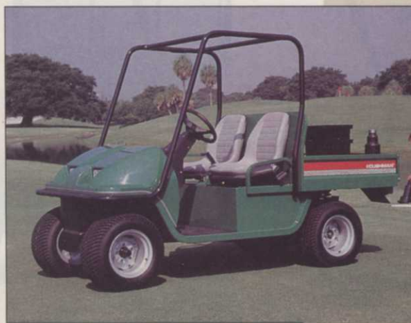
The Cushman Hawk comes equipped with a 50-amp alternator for running electric tools.
