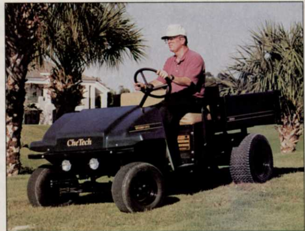
The Che Tech Groundforce 150 is equipped with an automotive style transaxle.
