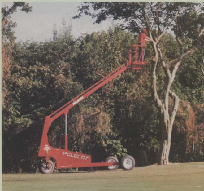
Operator-driven, self-propelled unit from Polecat Industries will not damage turf or landscapes. The lift is hydraulic.
