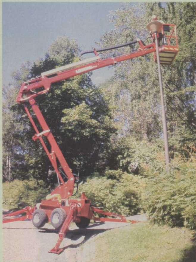
The Leguan Plus from Speciality Equipment has a 36-ft. working height, flexible aerial work platform, 298 lb. platform capacity.
