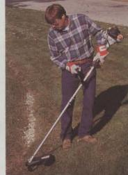
The Echo SRM-2100SB can function either as a line trimmer or blade brushcutter. Then, due to its split-boom design, it can be easily converted to an edger or other tool with optional attachments. The unit features a 21.2cc, dual-ring, piston engine with Pro-Fire electronic ignition backed with a lifetime ignition-module part warranty. Unit includes vibration-reducing handles and engine mount and a see-through fuel tank.
