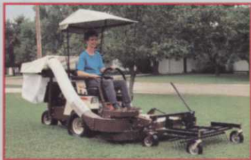
Durable 48- and 60-inch Tine Rake™ dethatchers remove thatch and surface aerate soil. Vinyl sunshade canopy protects operator from sun and heat.
