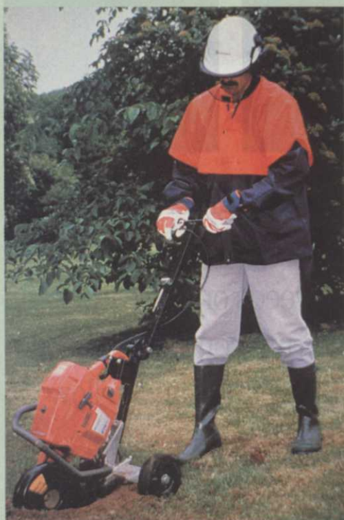
Husqvarna's 272S is a lightweight stump grinder with an 8-inch steel blade and anti-vibration technology. It folds and stores compactly.
