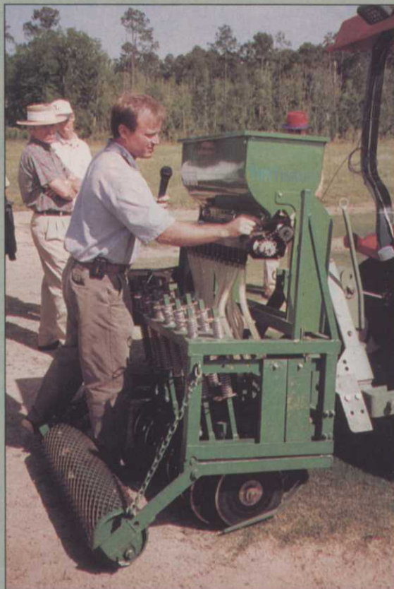
This machine makes slit applications at about a half inch below the soil surface.
