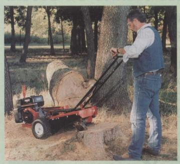
One of two models from Mackissic, Inc. Both with reversible handle bars. Automatic, self-aligning cutter head-to-shaft. Units require only two inches of clearance from walls, fences, trees.
