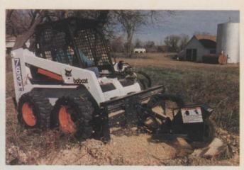
The SG50 stump grinder with the 763H Bobcat. Its 3-inch wide cutting head has 34 teeth, and cuts down 20 inches below grade.
