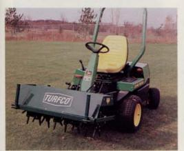
front rotary mowers. You can aerate right through tight turns with the tine wheels mounted separately in sets of two with greaseable oilite bearings. A heavy-gauge doubles as a weight tray to hold additional weight. Call Turfco Mfg. at (612) 785-1000, or
