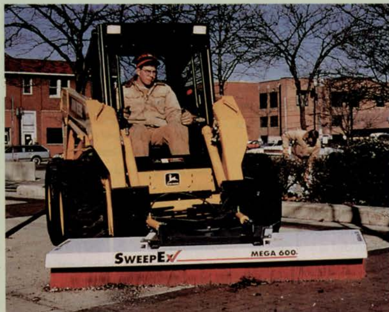
SweepEx Mega Series features 11 brush rows on 48-inch or 60-inch frame.
