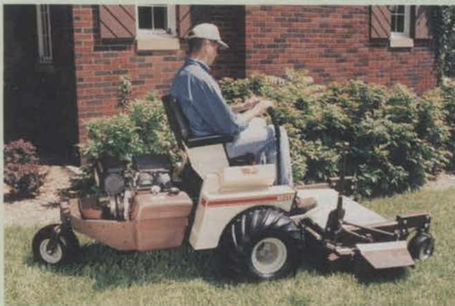
Grasshopper: outfront decks reduce secondary trimming.
