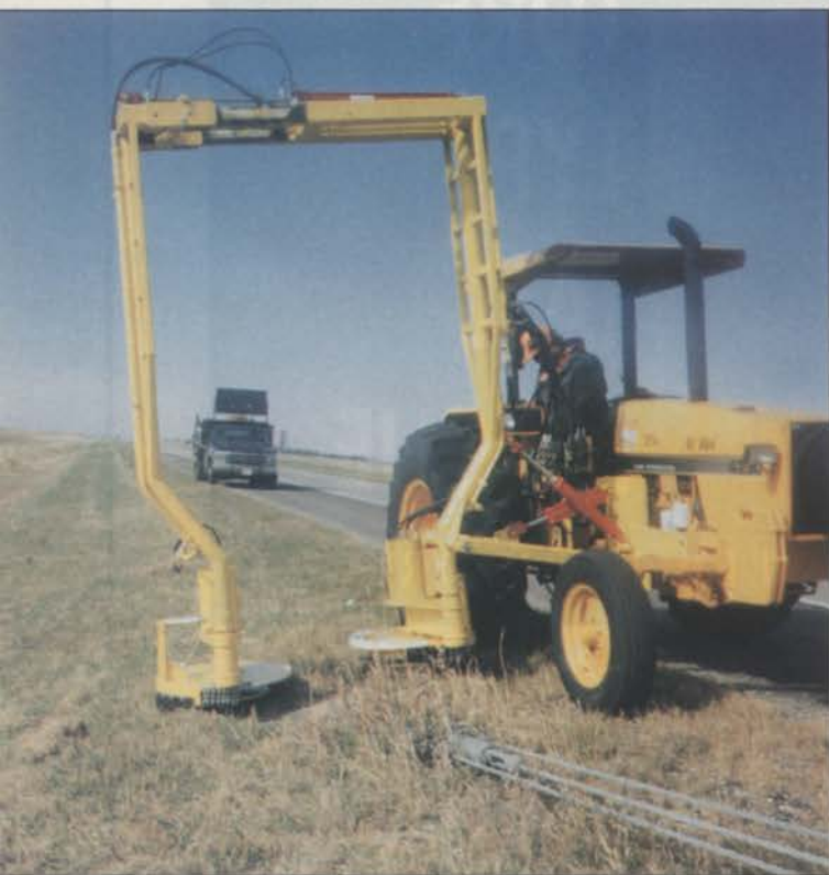
The Polecat mows around poles and on both sides of roadside structures. They're already being used in California and Colorado.
