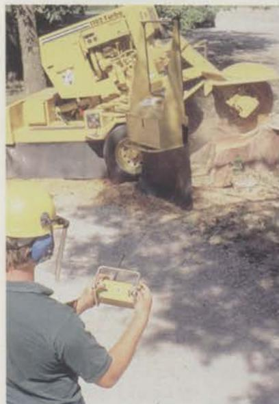
Vermeer Manufacturing Company offers wireless remote control for its stump cutter line. The radio remote control system option provides the operator more flexibility when positioning the machine in tight areas, and freedom of movement in an operating range of up to 100 feet from the machine. Currently available on the SC 1102 and SC 502 gearbox-driven stump cutter with Vermeer's Auto Sweep feature.
