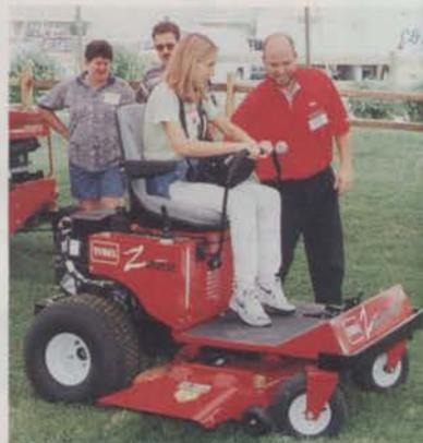
mand vertical shaft engine. The Z325 has a 25-hp Kohler Command vertical shaft engine. With a forward ground speed of up to eight miles per hour and a reverse speed of four miles per hour.
