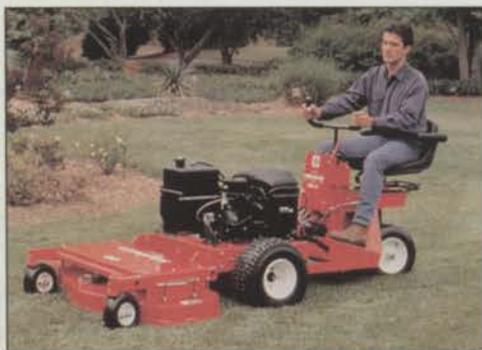
and comes with either a 50-inch or 60-inch mower deck. Hydraulic lift is standard equipment which allows easy maneuvers over curbs and other obstructions. Placement of the steering yoke and instrument panel permits operator almost unlimited visibility across the mower deck.
