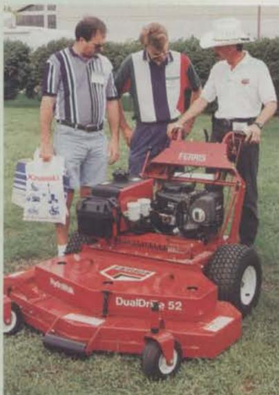
exclusive, dual-point floating front end. Two mounting joints in the front axle allow vertical travel at each wheel. The company says the mower will provide an unbeatable cut on uneven terrain.
