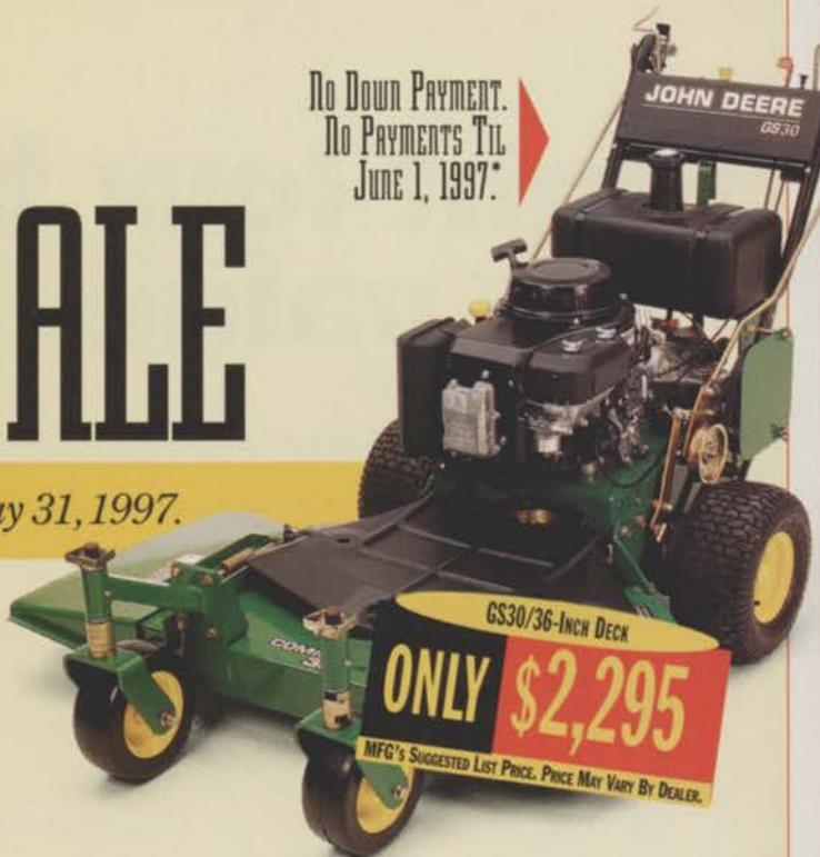
GS Series commercial walk-behinds are built to last. And with a new everyday low price, the 36-inch GS30 is as easy to own as most lesser spec'd mowers. You can mix and match overhead valve power units (13, 14 and 17 hp) with 36-, 48-, and 54-inch decks. Five-speed gear transmission with reverse. Knee- or hand-operated shift lever.
