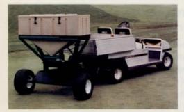
Grotech's MPS-125 is a multi-purpose, multi-season spreader. Spread seed, fertilizer and granular chemicals on turf in season, then turn the MPS-125 to winter maintenance, spreading ice melt and sand on your parking areas when the weather turns cold. This spreader also
