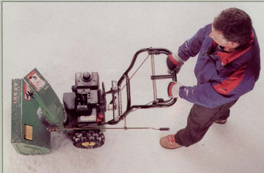
John Deere TR522 powered by 4-hp Tecumseh. Model 828 D has 8-hp engine and clears 28-inch path through the snow.
