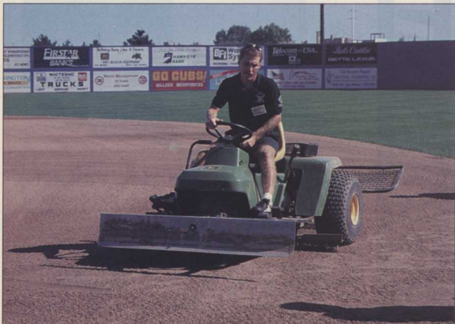
The scarifier located under the middle of this motorized field rake does a good job of working up the skin portion of a baseball infield, particularly the area around home plate.
