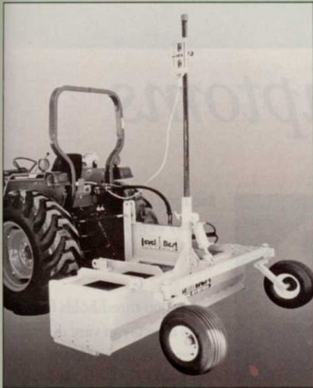
Level Best Grading System consists of grader box, laser transmitter and tripod, laser signal receivers, and an on-board control panel.
