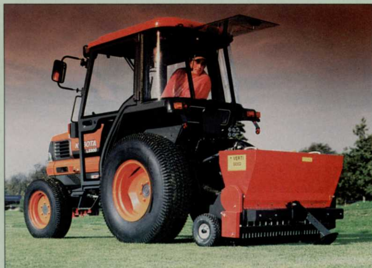
Verti-Seed overseeders in models with 34-inch and 50-inch working-widths. Compatible with tractors with at least 17 hp.
