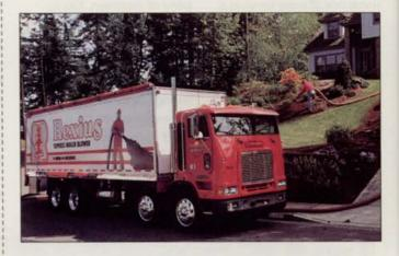
can blow any organic material up to 35 or 40 lbs. per cu. ft. with a particle size of approximately 3 inches and less. This includes decorative bark, sawdust, wood shavings, compost materials and wood mulch. Rate of application is 55 cu. yds. per hour. A 340-foot hose is included with the blower.
