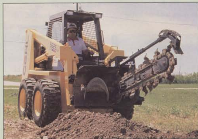
Gehl trenchers feature a heavy-duty digging chain.
