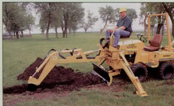
Vermeer increased the productivity and versatility of its V-3550 riding trencher with the addition of a backhoe.
