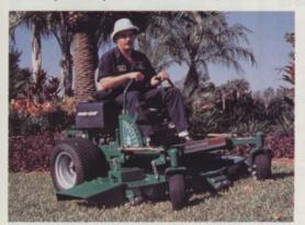
shrubs and small turf areas. Easy access to the cutter deck, belts and hydraulic reservoir makes service a snap. The wide stance of the tires enhances performance on hillsides.
