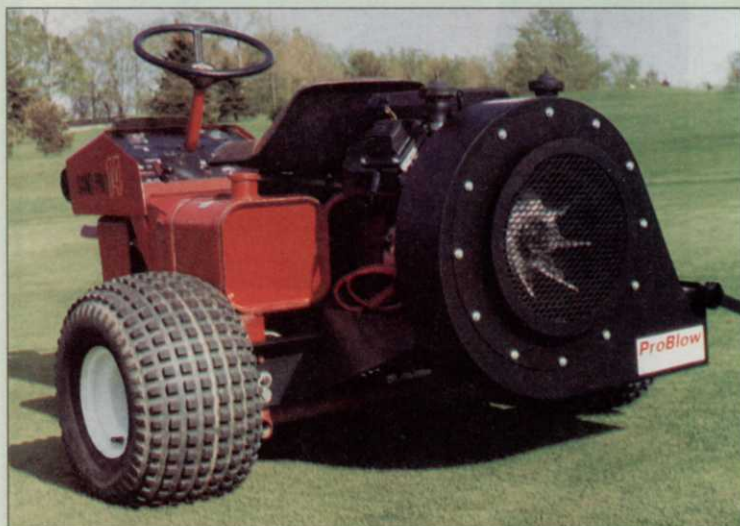
Selbro Pro-Blow mounts to Walker ZTR mower.
