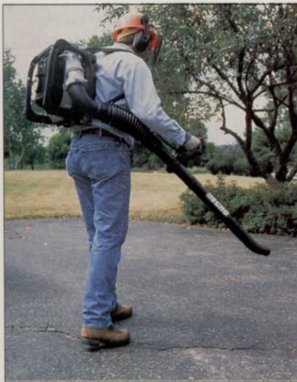
Echo PB4600, with tube-mounted throttle.
