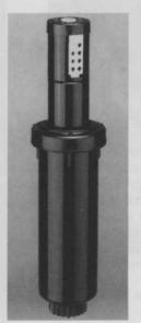
sprays water simultaneously from up to seven uniquely-engineered ports. With a simple turn of a screwdriver, flow can be set from 1 to 9 gal./min. The TruJectory system adjusts spray trajectory from 7 to 25 degrees without interrupting the water stream.
