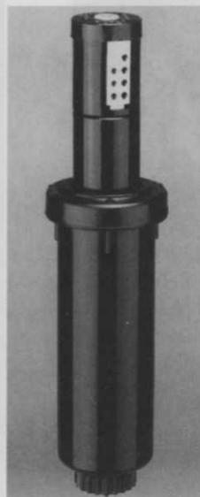
sprays water simultaneously from up to seven uniquely-engineered ports. With a simple turn of a screwdriver, flow can be set from 1 to 9 gal./min. The TruJectory system adjusts spray trajectory from 7 to 25 degrees without interrupting the water stream.
