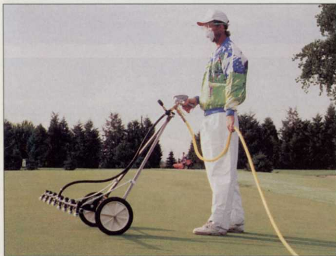
Broyhill's walking boom features an Accuspeed speedometer and an optional, 'see-through' drift cover.
