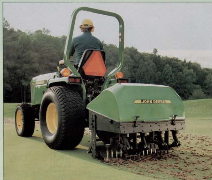
◀ John Deere Aercore delivers a 4-inch core.
