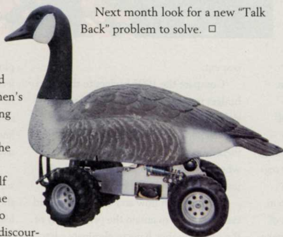
Jim Carpenter's Barberton, Ohio, crew constructed a radio-controlled 'Robo Goose' on a toy car chassis.
