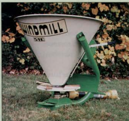
Vandermolen's Windmill spreader, above, has an effective spreading width of 40 feet. At left, the Gandy drop spreader can be used as a walk or tow unit.
