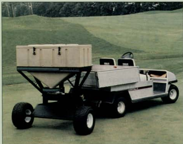
The Grotech multi-purpose spreader has universal mounts.
