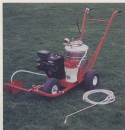
There's less refilling with Pioneer's Brite Striper 2000. It carries a 12-gallon tank.
