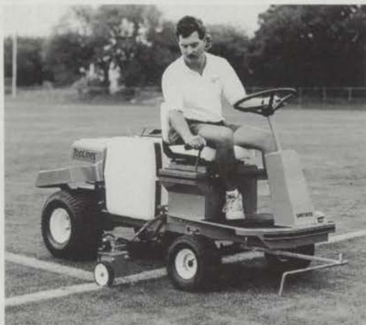
Smithco's Top Liner can be fitted with an optional hose and spray gun kit for paint or weed control spraying.
