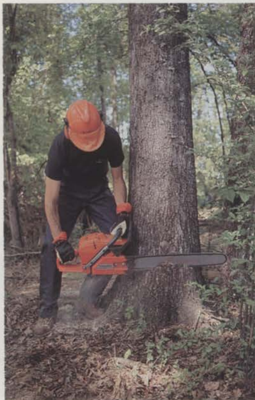
Be sure that the open notch cut is 70 degrees or more, to allow the hinge to guide the tree as it falls.
