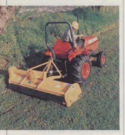
The vertically-rotating knife action of the flail mower projects the cut material downward into the grass, rather than out from under the mower. The AT60 and AT74 have cutting widths of 60 and 74 inches, respectively. Both are available in forward or reverse rotation.
