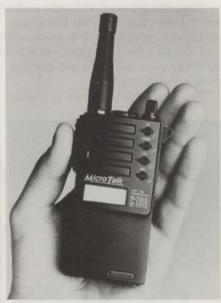
MicroTalk, which is the approximate size of a king-size cigaret box, is a five-watt, 10-channel synthesized radio featuring user-selectable scan to lock out or avoid busy channels. It is available in 148-174 MHz and 450-470 MHz frequencies.
