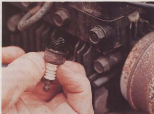
Late fall is the best time to change the oil one last time and check the spark plug.
