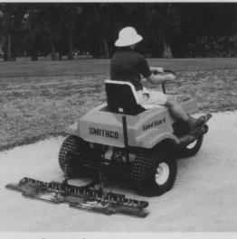
high-backed operator seat with a presence safety switch.
