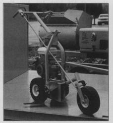
With a few passes, you can control the depth and width of a trench around existing flower beds, next to foundations, under fences and through grasses.
