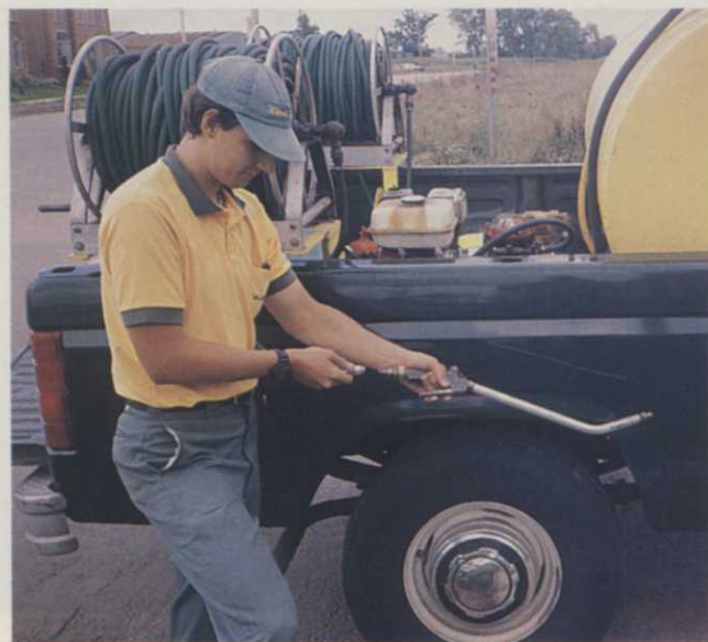
Quick couplings on spray guns help eliminate pesticide drips at the press of a button.
