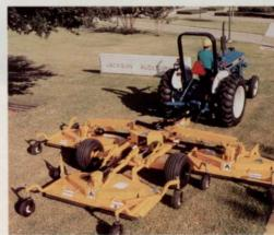
Small, highspeed blades allow rotary mowers to be used in fine turf mowing.
