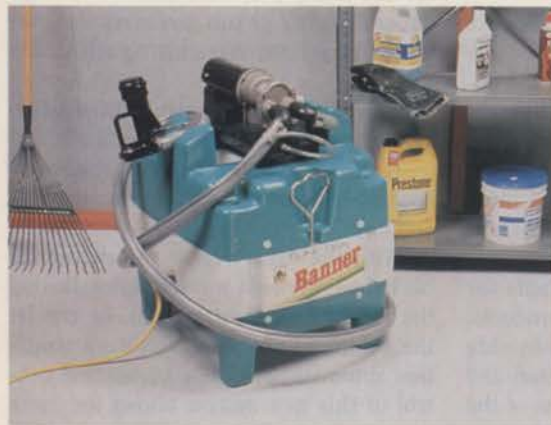
The 'turfPak' system as designed by Ciba limits pesticide exposure, speeds application time and ends package disposal problems.
