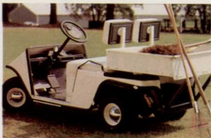
Melex 252 with solid state speed control
