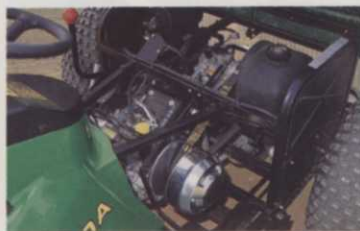
The 1200A now features the same engine and transmission found in the John Deere 4x2 Gator Utility Vehicle.
