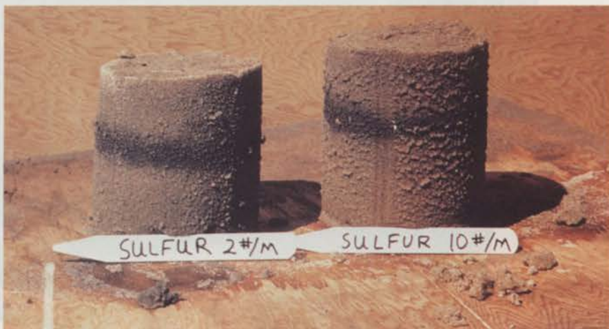
Black layer is a form of sulfur that has bonded with metal.
